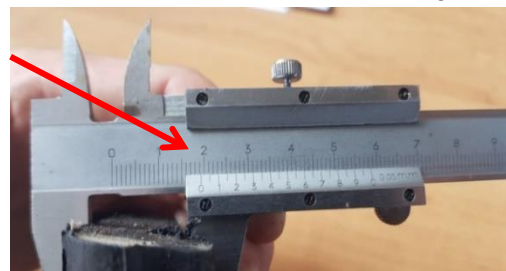
Fig. 6. Result of measuring the side surface of the coupling at the fastening place
