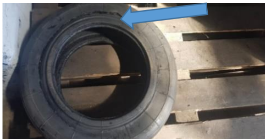
Fig. 3. ER2T 2207-02 damage to the side surface of the ER2T 2207-02 motor car rubber cord
