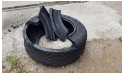
Fig. 4. Preparation of the rubber cord coupling for measurement
